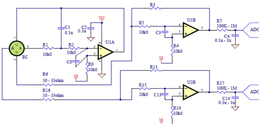
Notes: 1) In this reference schematic, VS and VR are reference voltages and should be short for the sensors with no bias voltage, such NO<sub>2</sub>, SO<sub>2</sub>, O<sub>3</sub> and CO sensor. It is recommended to set VS=VR=1.5V. 2) For the sensors with bias voltage, such as NO(bias +300mV), it is recommended to set VS-VR=300mV
